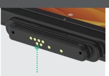
Flush, easy to clean charging contacts provide port protection, seamless high-speed charging, and compatibility across the GDS<sup>®</sup> Ecosystem<sup>™</sup>
